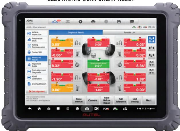
Employing 6 HD position and tracking cameras, the IA900WA performs precise four-wheel alignments to 0.02 degrees of accuracy. Step-by-step instructions guide the technician through the complete process with illustrated, color-coded alignment status, live readings, required tools.
